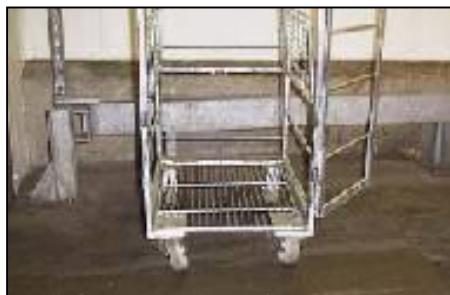
Wheels bent so trolley is unstable
