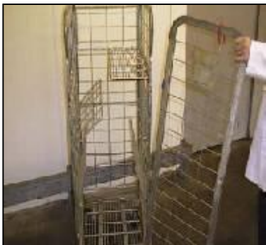
Door, frame, hinges bent or missing
