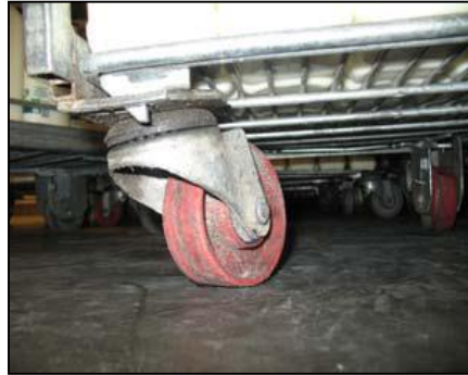
Broken wheel plate
