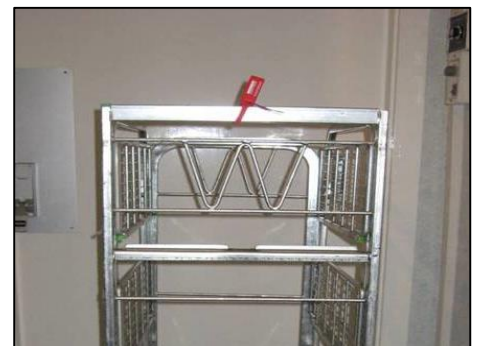
An example of a red tag system to indicate a damaged trolley
